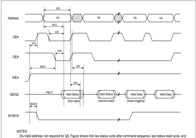
VA=Valid address; not required for Q6. Figure shows first two status cycle after command sequence, last status read cycle, and array data read cycle.
