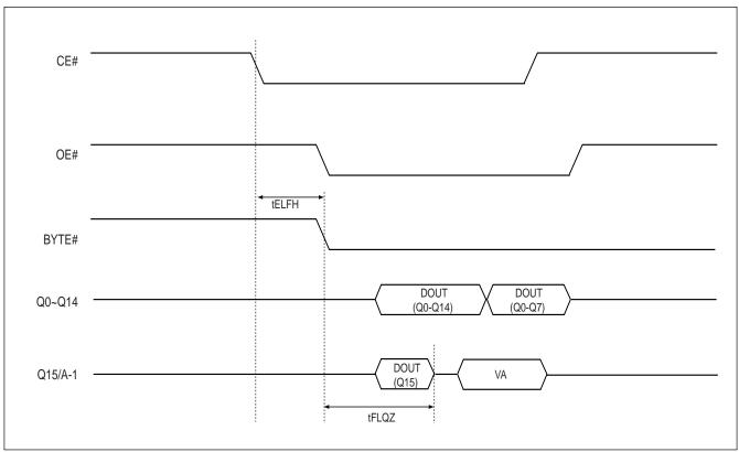
Figure 25. BYTE# TIMING WAVEFORM FOR PROGRAM OPERATIONS
